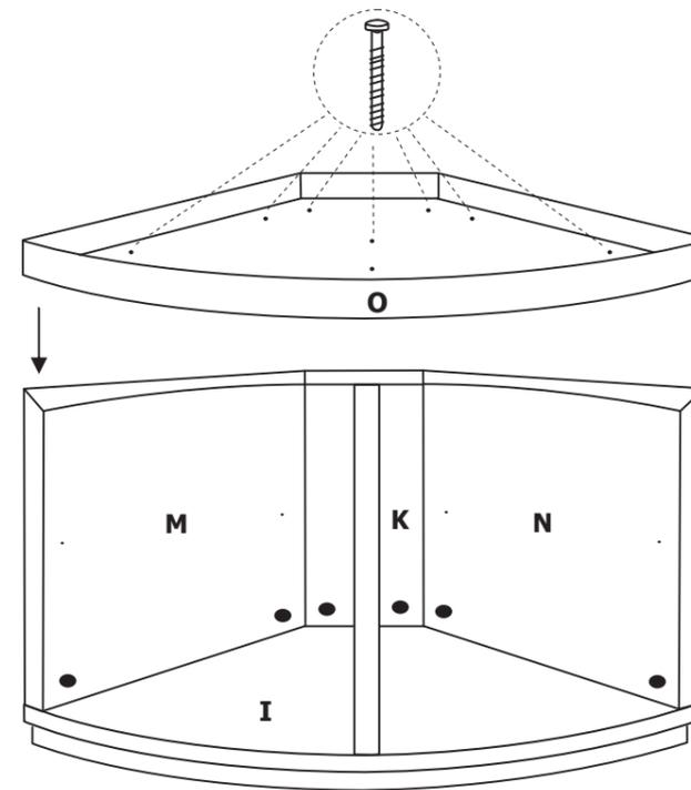
Position cabinet lid on the cabinet construction, open side pointing upwards. Line up screws C with holes and fasten, ensuring screw heads do not stand proud.
