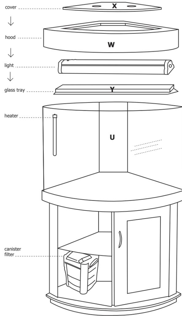
Place aquarium **U** on top of cupboard **by lifting it on from the back and sliding it forward.**
