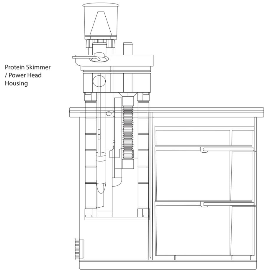
5. Connect the Small piece of flexible hose to the Outlet of the Power Head and position the Power Head in the housing. Feed the power cord through the side of the housing.
