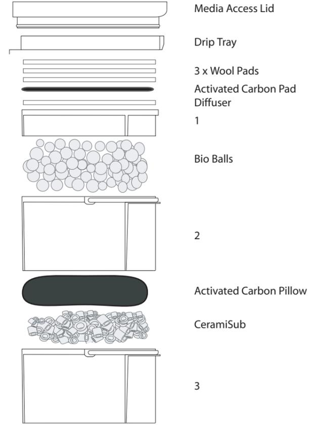
3. Remove Carbon Pillow and CeramiSub from their plastic bags. Wash all media under clean tap water and place all media back into the Media Baskets and back into the Filter Box. Do not replace the Drip Tray or Media Access Lid.
