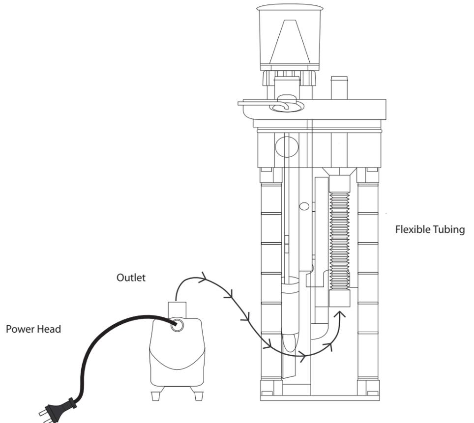
6. Slide the Housing back into the Filter Box, ensure the power cord from the Power Head is fed through the Power Head Cut out. DO NOT force the Housing in. Remove and try again.
