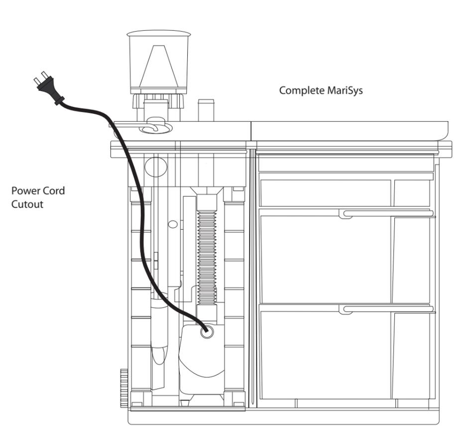
7. Place the complete MariSys under the aquarium. Hang the Overflow Box on the back or side of the aquarium. Measure and cut Hoses to length. Allow a little slack. Place Hose Clamps over the end of the Hoses and connect them to both the Overflow Box and MariSys and tighten.
