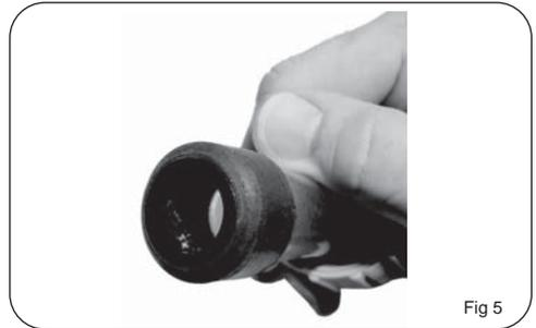
8. Then insert the hose end with the grommet on it into the inlet/outlet. Fig6
