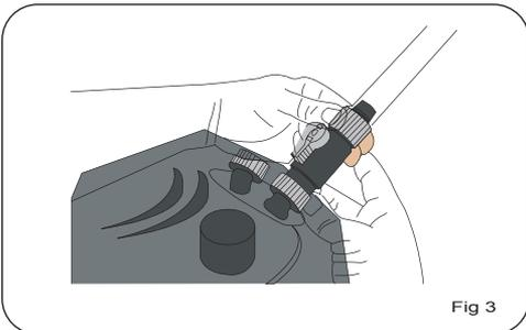
5. Be sure not to cross thread the tap as this may crack the seat and cause it to leak. Over tightening the tap will have the same effect. **NO TOOLS ARE REQUIRED. HAND TIGHT IS ENOUGH.**
