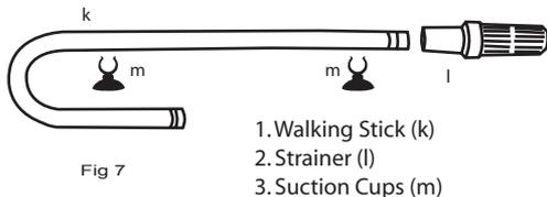
15. You will notice in your accessory boxes an extension for very deep aquariums. Attach the extension onto the bottom of the Walking Stick (k) then the Strainer (l) onto the bottom of the extension.
