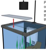
Place the lids on the top frame as shown. Place the larger lid at the back.
