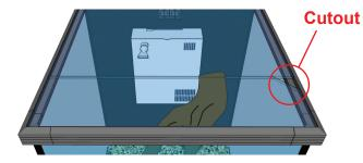
Position the front lid with the cutout in the location desired. This may be used both as a feeding hole and also to make it easier to remove the lid required.
