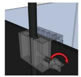
Position the light at the desired height and tighten the locking screw.
