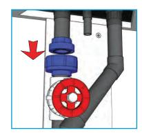
Remove the gate valve assembly.
