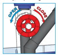
Set the gate valve to around the middle position (around three turns from fully closed) and start the return pump.
