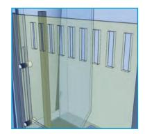
Check the grille on the movable baffle for blockages. If only part of the grille allows water through, it can become noisy.
