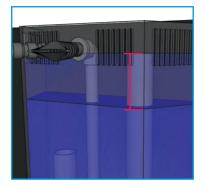
Check that the drain system is functioning correctly (it should be silent) and that water is flowing through the aquarium properly.
