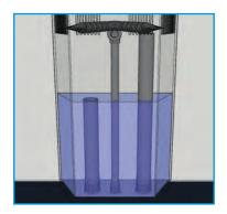
Check the water level in the weir. If the level is too low, air will be drawn into the main drain creating the sound.
