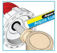
Lubricate the internal thread and o-ring of the gate valve.
