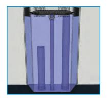
If the level is too high, water will spill into the emergency drain, drawing air into it creating the sound.
