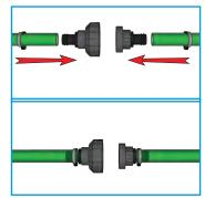
Connect the return hose to the quick connect coupling. Use hose clamps to secure the connection.
