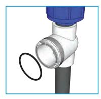
Remove o-ring from the valve body.
