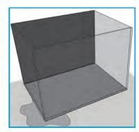
If the water level has dropped, there may be a leak in the tank body itself. To find a leak, it may be necessary to remove the tank, dry it and place it on newspaper to find the leak.
