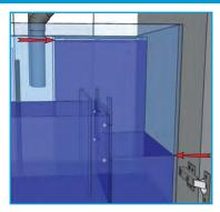
Check the water level in the sump. If you are using an automatic topup system, ensure that the ATO reservoir has enough water.
