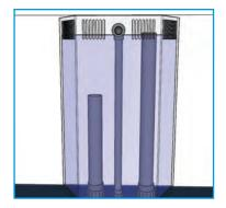
Repeat this procedure until the water level in the weir is just below the emergency drain. Once the correct setting is found, it should require little attention but may need adjustment from time to time.
