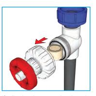
If adjusting the gate valve doesn't affect the water level, there may be a blockage in the main drain.
