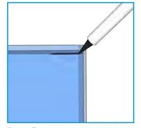
Turn off all pumps and mark the water level with a marker. Leave the tank for at least a few hours and see if the water level has dropped.
