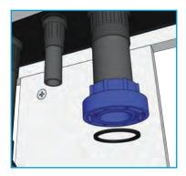
Remove o-ring from the barrel union body.
