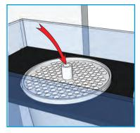
Check that water is flowing through the filter sock correctly. If it is clogged, the water will spill over the silencer overflow shown.
