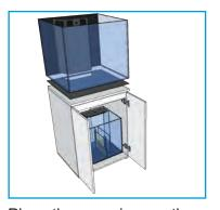
Place the aquarium on the cabinet. Ensure that the Foam Base is in place.
