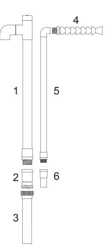
4. Ensure the sump is on the far left hand side of the cabinet so that the drain pipe sits directly over the sump inlet. Attach the bottom section of the drain (3) by connecting the barrel union.
