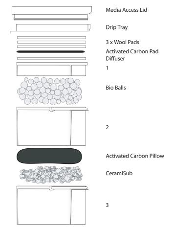
3. Remove Carbon Pillow and CeramiSub from their plastic bags. Wash all media under clean tap water and place all media back into the Media Baskets and back into the Filter Box. Do not replace the Drip Tray or Media Access Lid.
