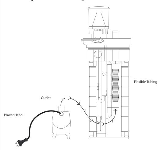
6. Slide the Housing back into the Filter Box, ensure the power cord from the Power Head is fed through the Power Head Cut out. DO NOT force the Housing in. Remove and try again.
