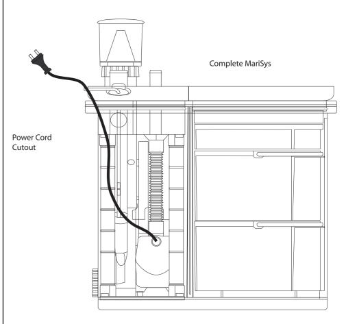
7. Place the complete MariSys under the aquarium. Hang the Overflow Box on the back or side of the aquarium. Measure and cut Hoses to length. Allow a little slack. Place Hose Clamps over the end of the Hoses and connect them to both the Overflow Box and MariSys and tighten.
