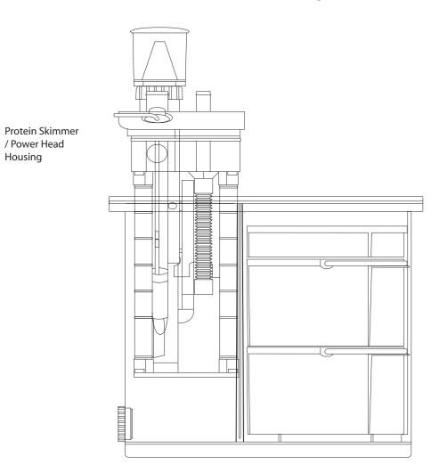
5. Connect the Small piece of flexible hose to the Outlet of the Power Head and position the Power Head in the housing. Feed the power cord through the side of the housing.
