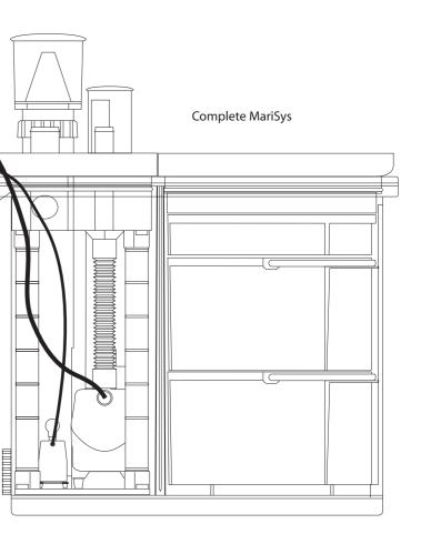
7. Place the complete MariSys under the aquarium. Hang the Overflow Box on the back or side of the aquarium. Measure and cut Hoses to length. Allow a little slack. Place Hose Clamps over the end of the Hoses and connect them to both the Overflow Box and MariSys and tighten.
