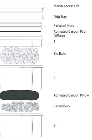
3. Remove Carbon Pillow and CeramiSub from their plastic bags. Wash all media under clean tap water and place all media back into the Media Baskets and back into the Filter Box. Do not replace the Drip Tray or Media Access Lid.
