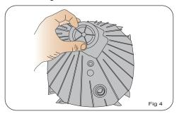
14. Then pull the impeller cap off and remove the impeller. Fig 5
