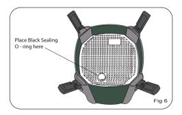
9. Prior to installing the head unit, turn it over so you can see the impeller. Make certain that the power cord is not wet and plug it into the receptacle then turn it on and ensure it is working. If the impeller does not turn see Cleaning Your Filter for instructions on how to assess the impeller. Remove the Black sealing O-ring from the feeder pipe. Fig 7 and place it on the filter inlet pipe on the top filter basket. Fig 6
