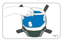
6. Follow the filter media setup instructions on the previous page which apply to your filter. Remember to remove all media from the plastic bags and rinse in tap water to remove excess dust. The simplest way to do this is empty the correct media into its basket and run tap water through it. Rinse the inside of the canister body in tap water. **DO NOT USE ANY SOAPS OR DETERGENTS.** Fig 4
