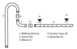
9. Attach a Joiner (b) on to the shorter side of the Walking Stick (a), insert an Elbow (c) into that. Then attach another Joiner (b) onto the other end of the Elbow. (c) Insert the Spray Bar (e) into the other end of the Joiner (b) . Press together firmly. Attach Suction Cups (d) to the Spray Bar.
