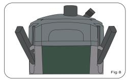
canister and the head unit. Do not force it together! If it feels tight do not apply any pressure to close it simply, remove the head unit and filter baskets and try again. Fig 8
