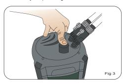
3. Depress all the way then release. Fig 4. Continue to pump the primer until the water flows down the inlet tube and begins to fill the canister.
