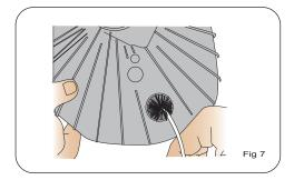
17. Pull the rubber end cap off the shaft of the impeller and run water through the hole in the middle of the impeller. Clean any debris which may have built up on the shaft off, along with any slime build up on the impeller. Fig 8
