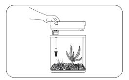
19. Place the light unit on the front of the aquarium, with the power cord passing through the light cord channel. Fig 3
