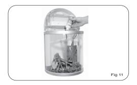
17. If you have installed the outlet with the spray bar (Option 2) attachment make certain the holes are not facing upwards.
