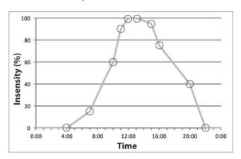
4. Light compensate: In light compensation mode, the degree of compensation can be adjusted. The value can be adjusted from 1-10. Higher values will increase the amount the intensity rises or falls relative to the ambient light.
